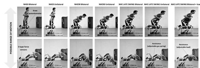
**Fig. 1.** Description of the Hamtech device main exercise modalities: Nordic Hamstring Exercise with extended hip (NHE0), Nordic Hamstring Exercise with 90° hip flexion (NHE90), Nordic Hamstring Exercise with sprint late swing phase kinematics (NHE Late Swing). Note that isometric testing can be performed at any of the possible hip-knee angles within that range of motion. See video in Supplementary material.
