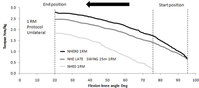
**Fig. 5.** Typical angle-torque profile for a football player, during a 1RM test in NHE0 exercise (light grey), in the NHE Late Swing mode (dark grey) and in the NHE90 mode (black). After calibration, start and end position angles correspond the actual anatomical knee angle (calibrated, as on an isokinetic machine) and not to the *Hamtech* frame angles.
