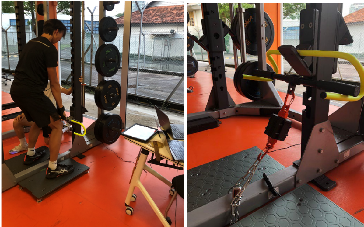
Fig. 1. “Open-chain” configuration of the isometric mid-thigh pull (IMTP) test.
